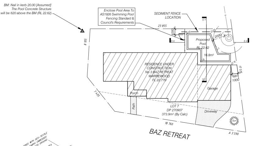
POOL OVERFLOW TO BE PUMPED TO SEWER TO COUNCIL'S & SYDNEY WATER'S REQUIREMENTS
