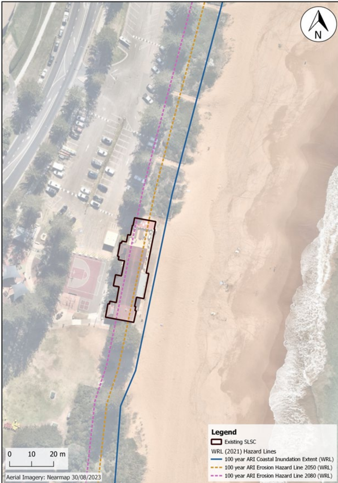
Figure 3-11 Revised Coastal Hazard Extents following implementation of secant piled seawall (after: WRL, 2021)
