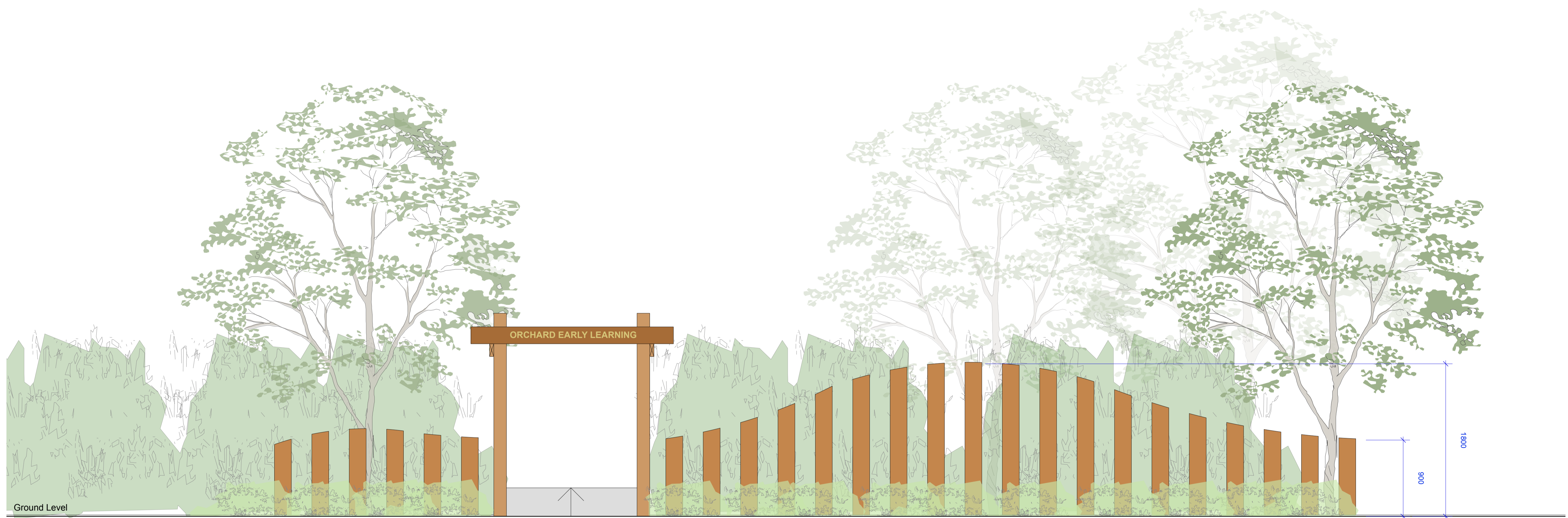
VERTICAL SLEEPER SCREEN ELEVATION 1:25
