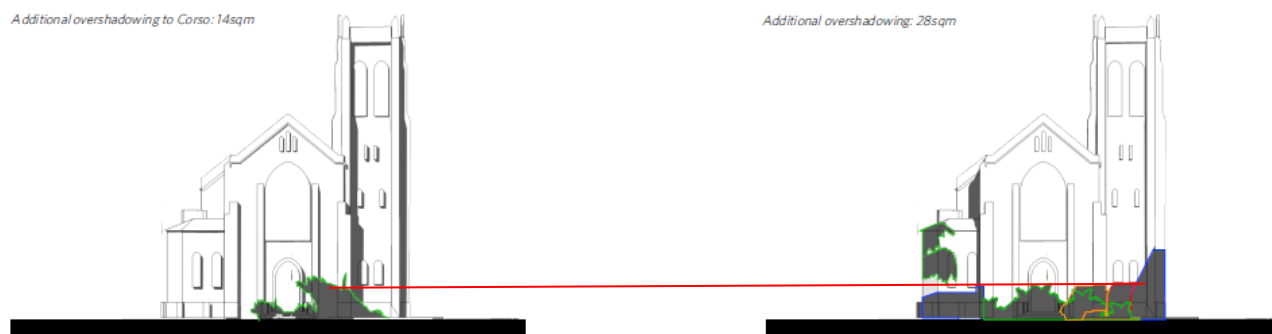
Figure 11: Elevational shadow diagram demonstrating impact of the proposed building height, as directed by the MDCP, on the existing window opening to St Matthews Church
