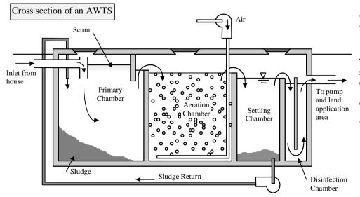
to assist bacteria to further treat it. A third chamber allows additional clarification through the settling of solids, which are returned for further treatment to either the septic chamber (as shown) or to the aeration chamber. The clarified effluent is disinfected in another chamber (usually by chlorination) before irrigation can take place.
