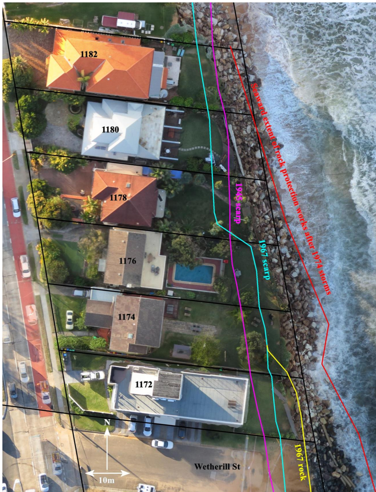
Figure 4: Erosion escarpment at subject properties after 1945 and 1967 storm, and extent of 1967 and 1974 rock protection works, overlaid on 8 June 2016 aerial photograph
