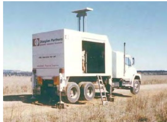
Figure 2: Purpose built CPT rig
