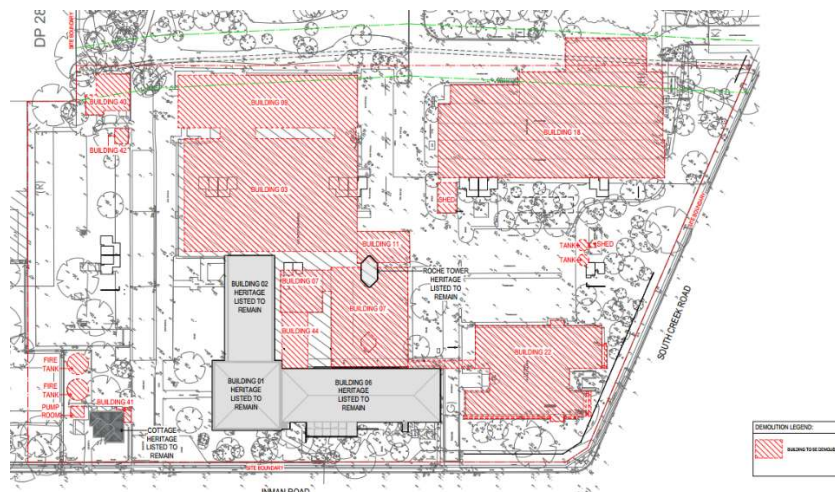
Figure 7: Approved Demolition Plan for the Northern Beaches Business Park DA 2019/136 showing the retained built elements of heritage significance. (Source: Northern Beaches Council DA Tracker website. Plan prepared by SBA Architects DA208 Revision 12 dated 12.11.2019)
