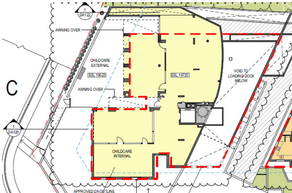
Figure 1 – Increase in setback of Building C to upper ground level (approved building footprint shown in red)
