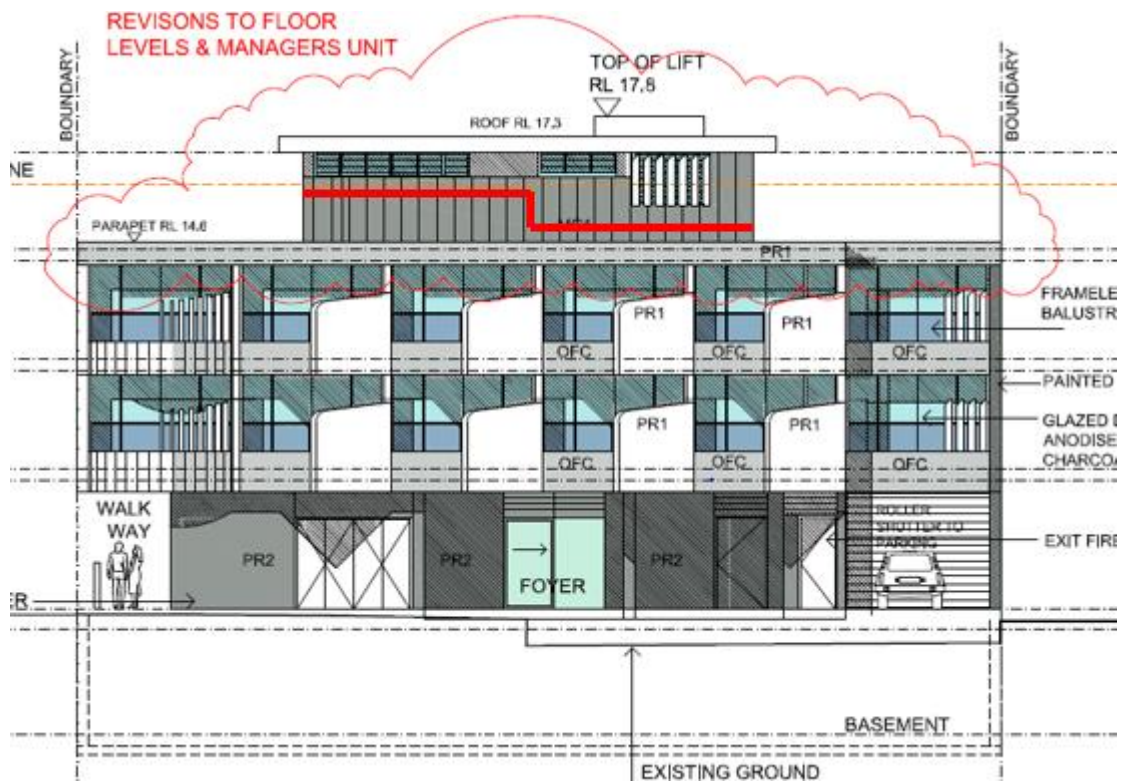
Figure 3 - Plan extract showing extent of 11 metre building height breach as viewed from the west (rear of site)
