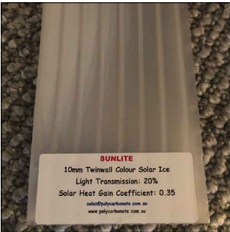
Polycarbonate roofing material. 10mm Twinwall Colour: solar ice
