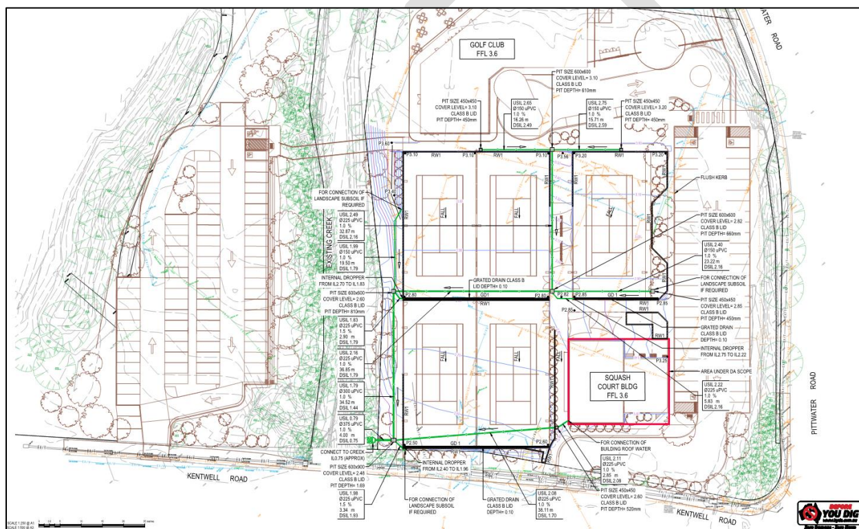
Figure 18. Stormwater Management Plan (Source: Acor Consultants, 2024)
