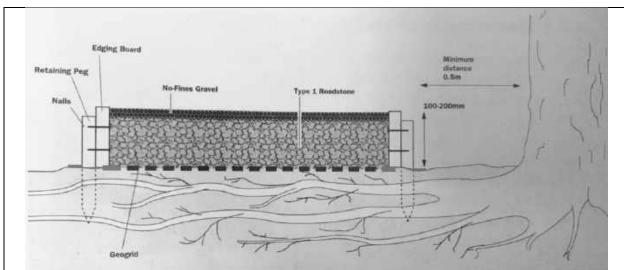
**Image A**: An image from 'Tree Roots in the Built Environment'<sup>9</sup>, showing how to construct a driveway above a trees root system without excavation. Type 1 Roadstones are an example of blue metal.
