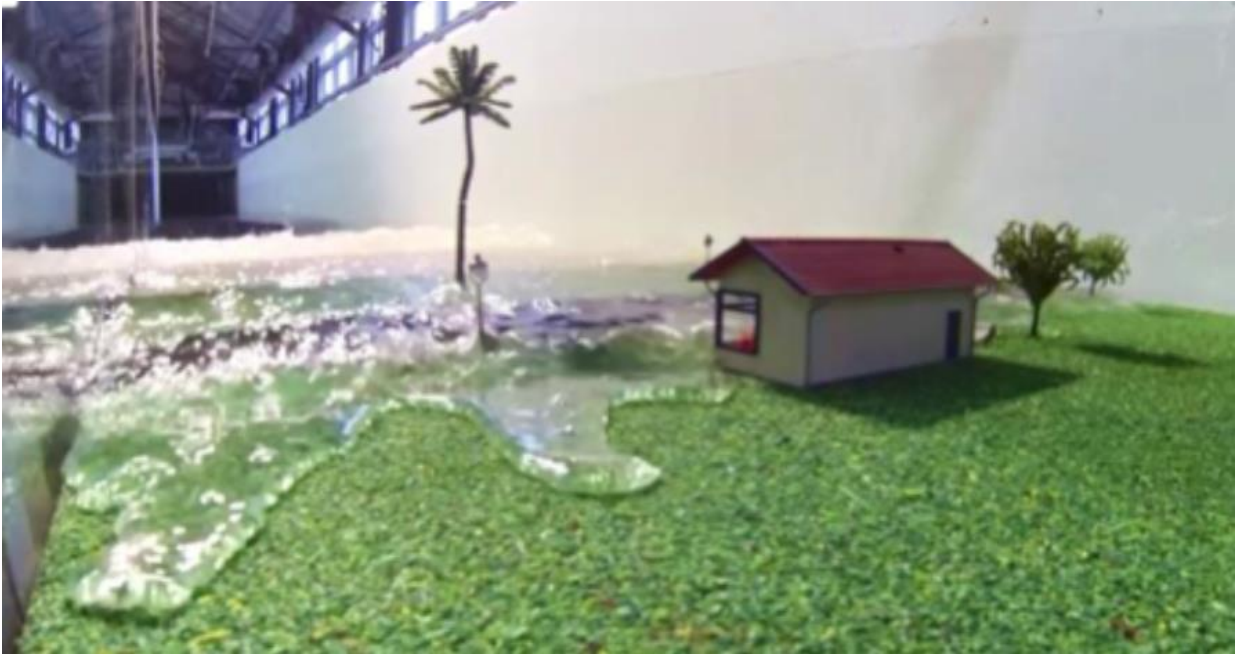
Figure 8: Example of physical model examining wave forces on a building
