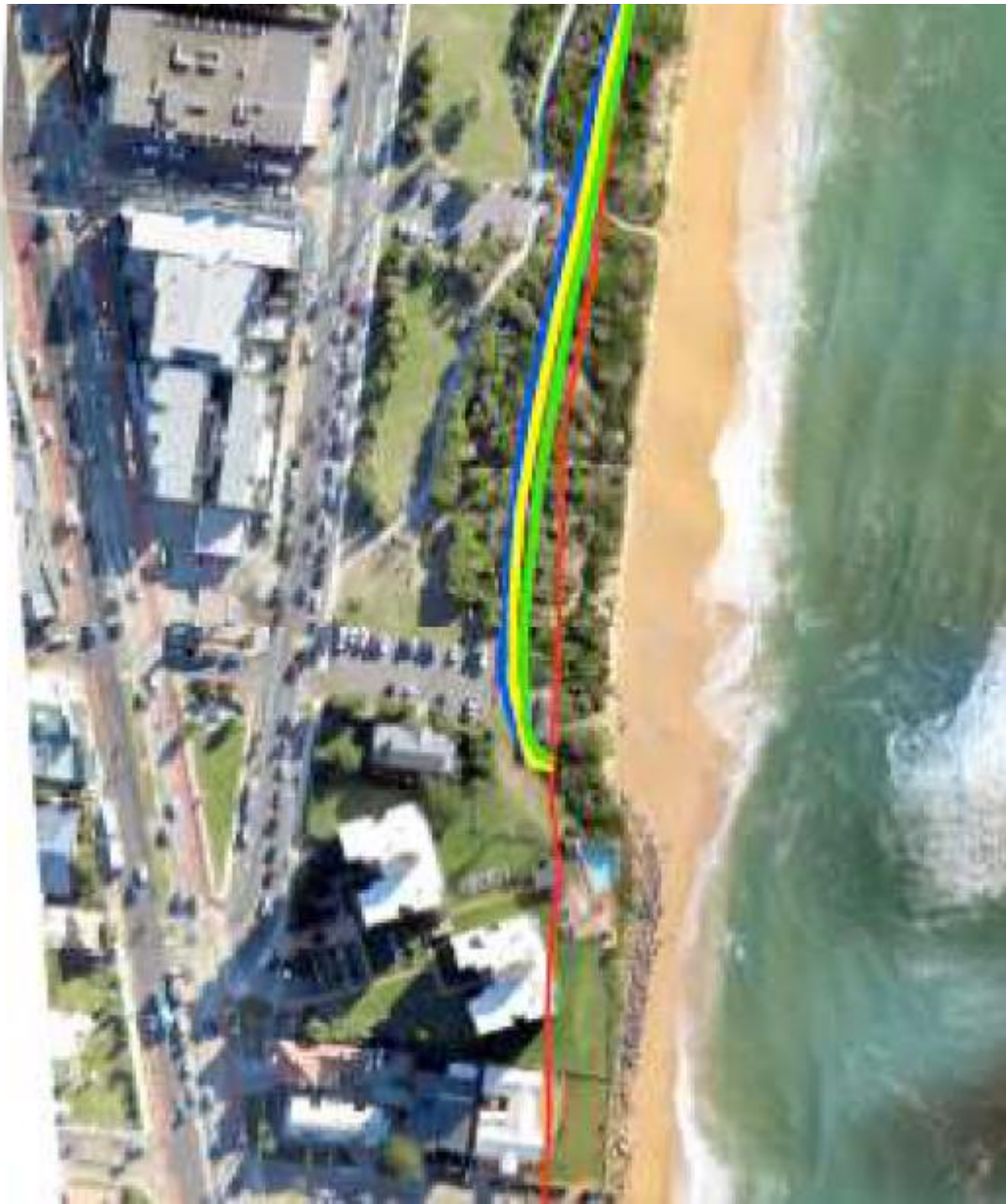
Figure 7: Example of calculated seawall end effect (red line is erosion extent without seawall)
