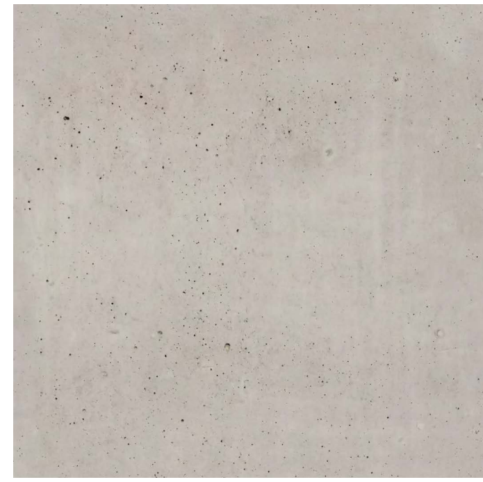
CONC NATURAL OFF-FORM CONCRETE
