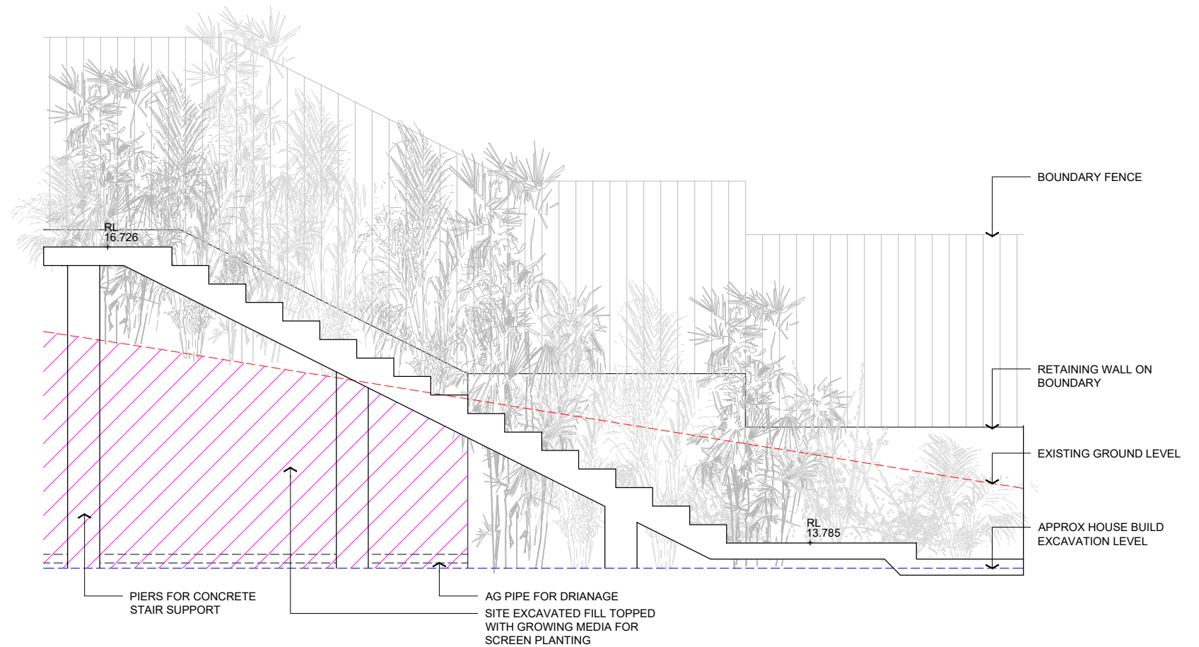
SECTION 05 (TYP) - ENTRANCE STAIR Scale: 1:50@A3
