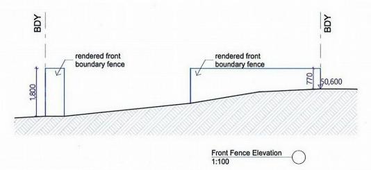
Sketch A: extract from DA drawings showing 1.8m high front fence. Southern 1.8m high fence to be reduced to 1m.
