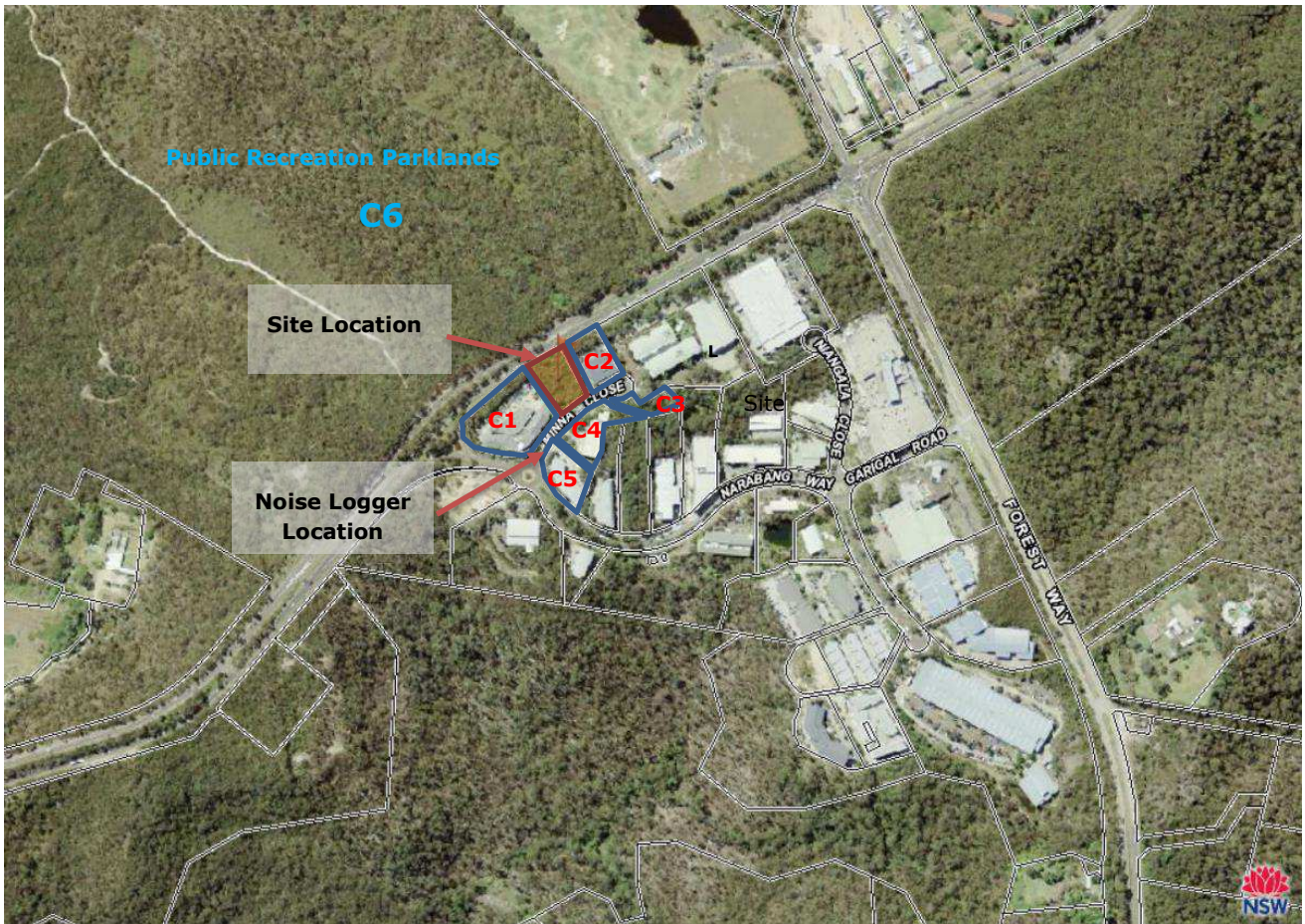
Figure 3-1: Site Map, Receiver Locations (C1 to C4) and Unattended Noise Logger (L) Location.
