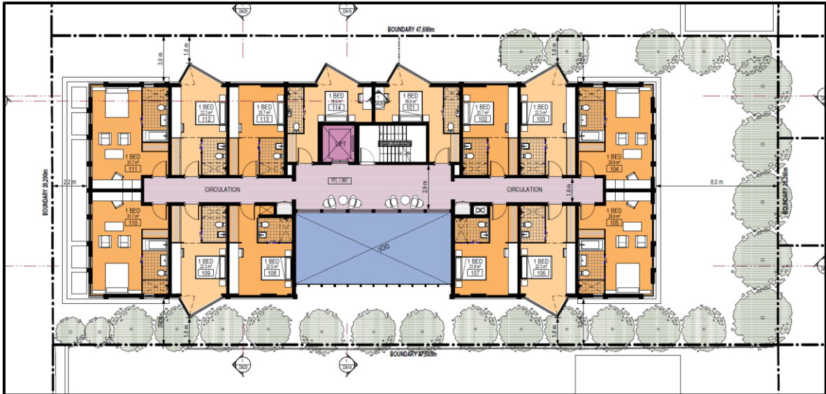
Figure 32: Proposed typical floor level of the building
