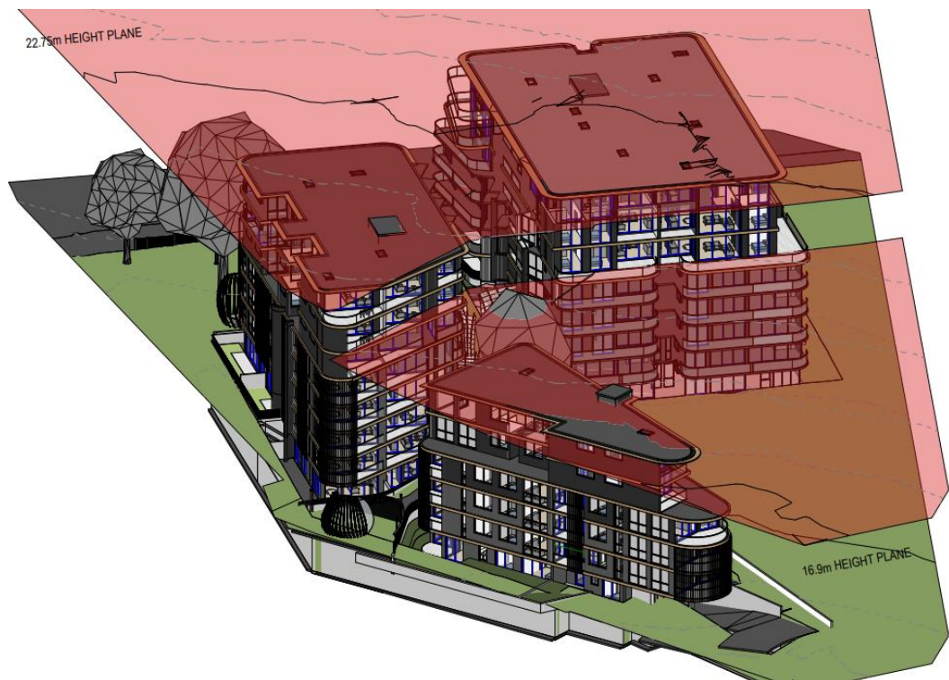
Figure 2 - Plan extract showing minor breaches to building height for Buildings B and C (source: Brewster Murray).
