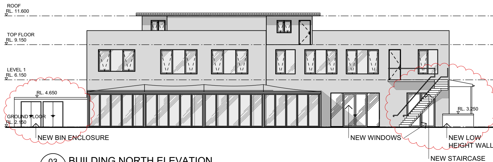
03 BUILDING NORTH ELEVATION scale 1:200
