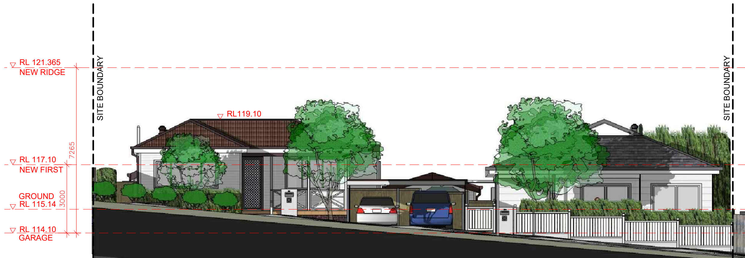
EXISTING WEST ELEVATION (STARKEY STREET)
