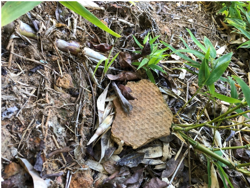
Photograph 8: Fibro-cement piece on the surface near EBH103 (18/06/2021).
