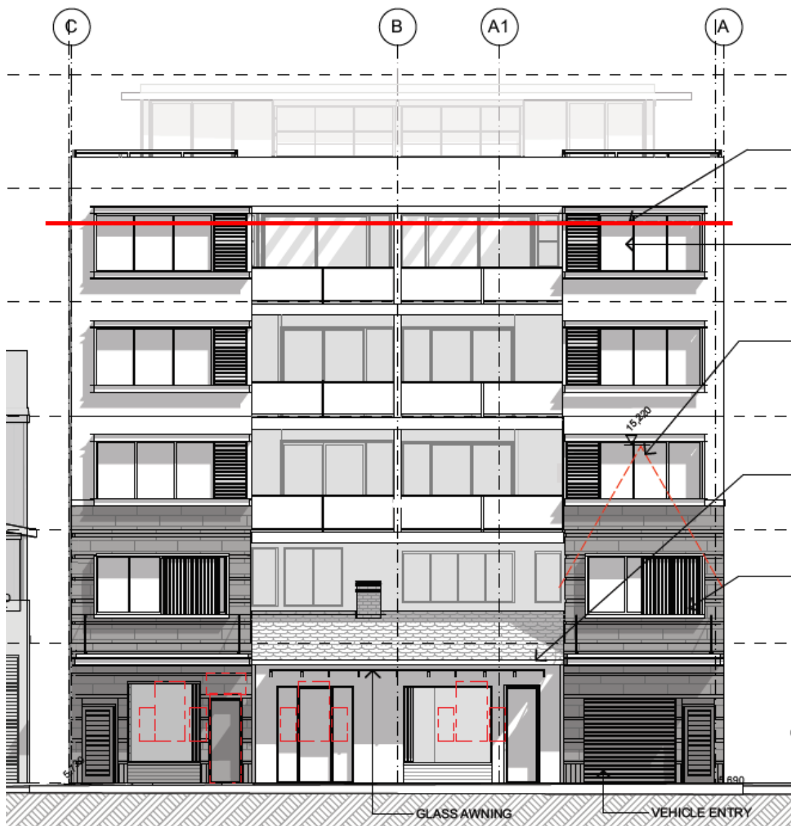
Figure 6 – Extent of building height non-compliance.
