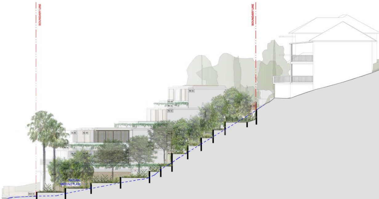
Figure 10 – Southern elevation plan extract showing the highly articulated and step nature of the building form proposed.
