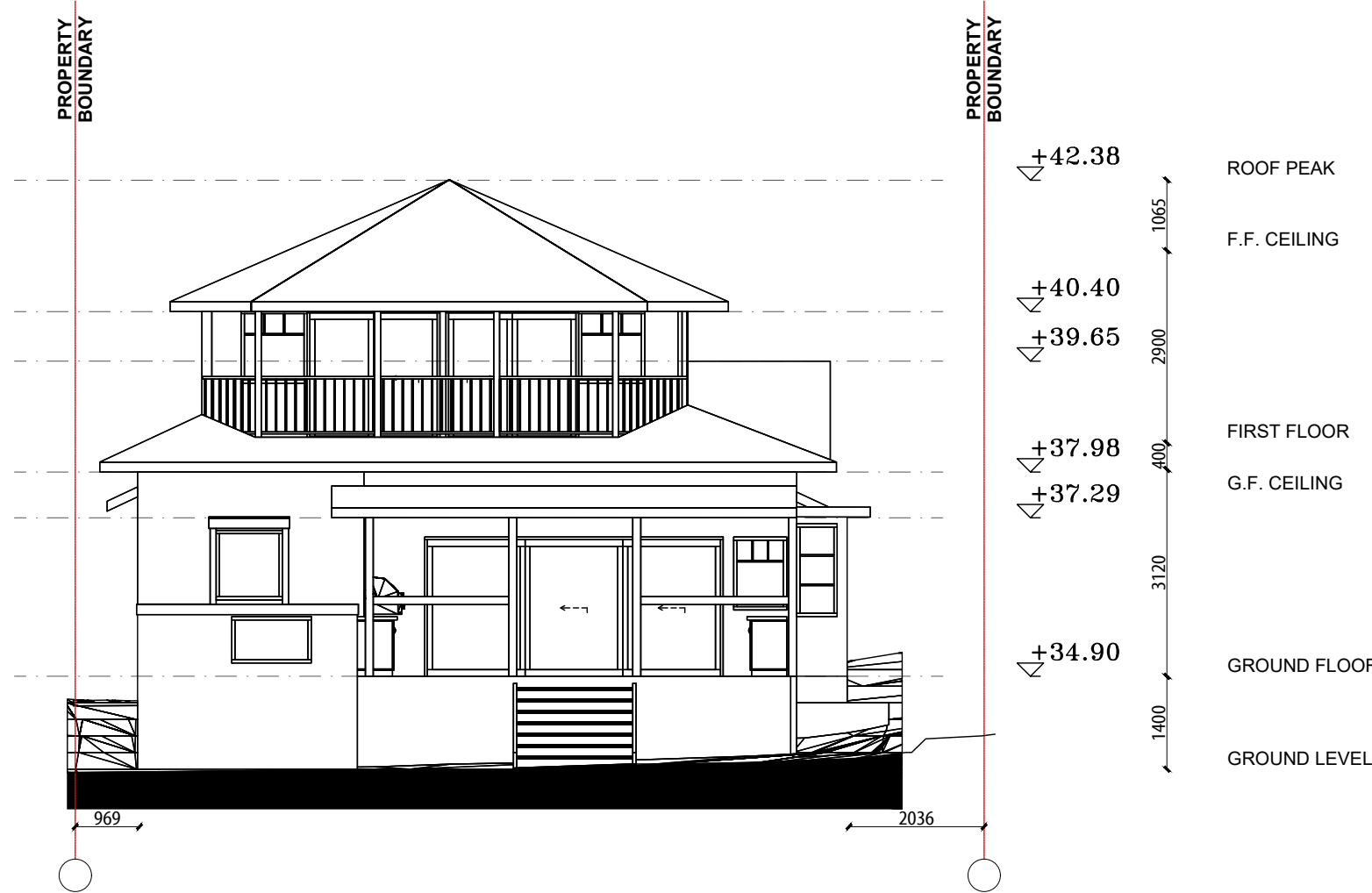
4 E-4 EAST ELEVATION - PROPOSED Scale 1:100
