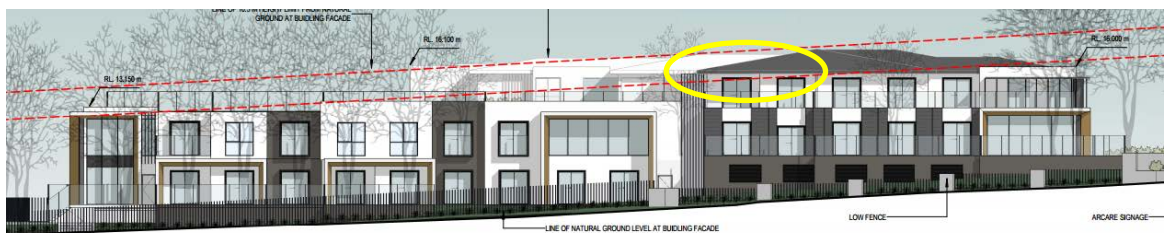
Figure 3 – Macpherson Street (southern) elevation with 8.5m and 10.5m height limit shown in red Source: V-Arc
