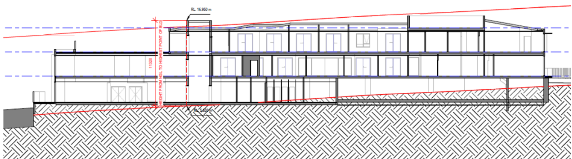
Figure 2 - Section through building with 10.5m height limit shown in red Source: V-Arc
