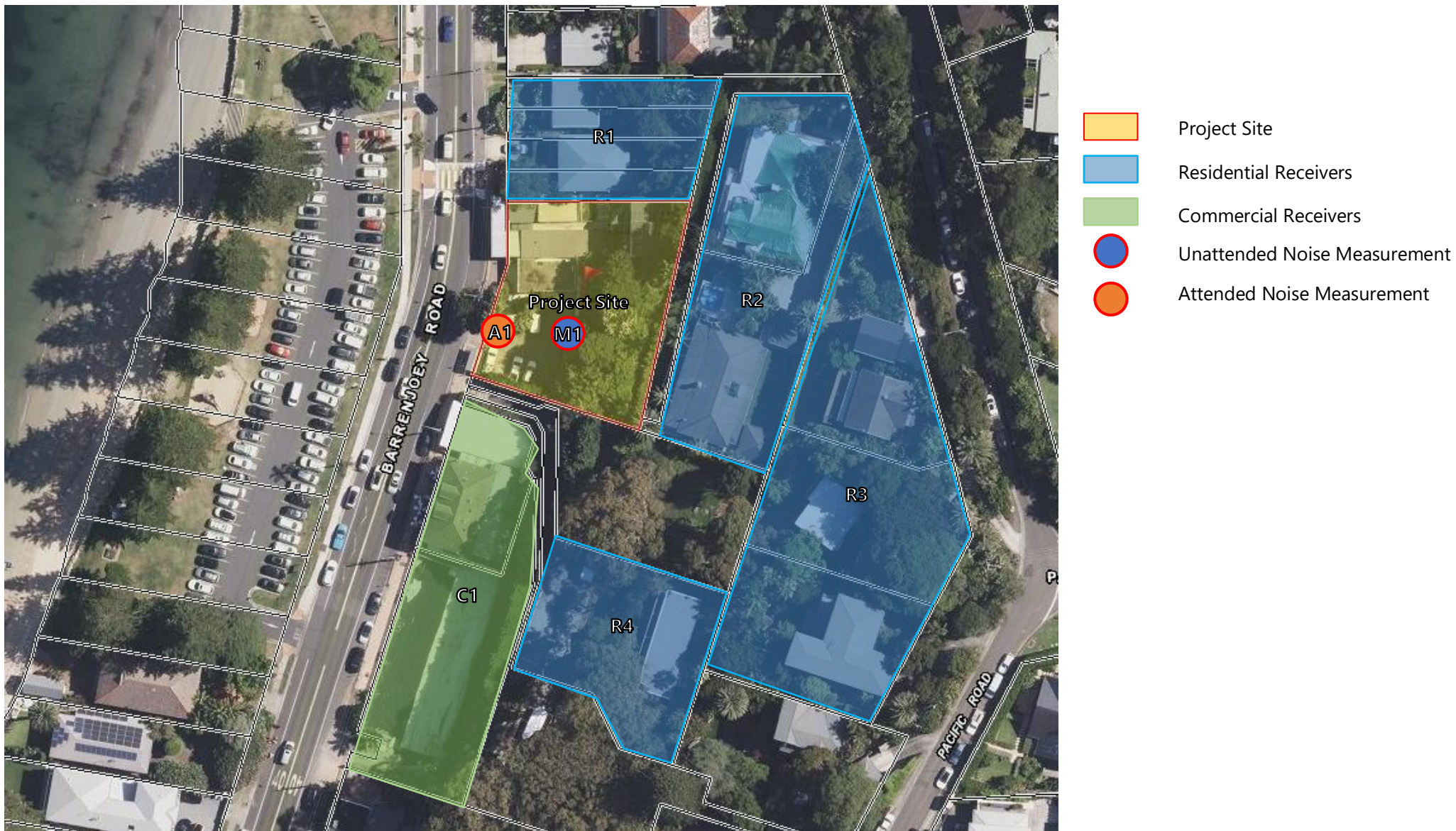
Figure 1 : Aerial View of the Project Site, Sensitive Receivers and Monitoring Locations.
