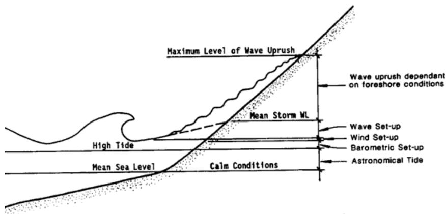
**Figure 12 - Components of elevated water levels on the coast (NSW Government, 1990)**
