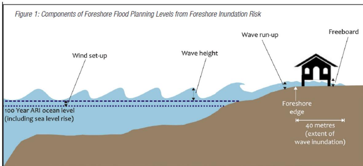
**Figure 10 – Components of the FFPL (Cardno, 2011)**
