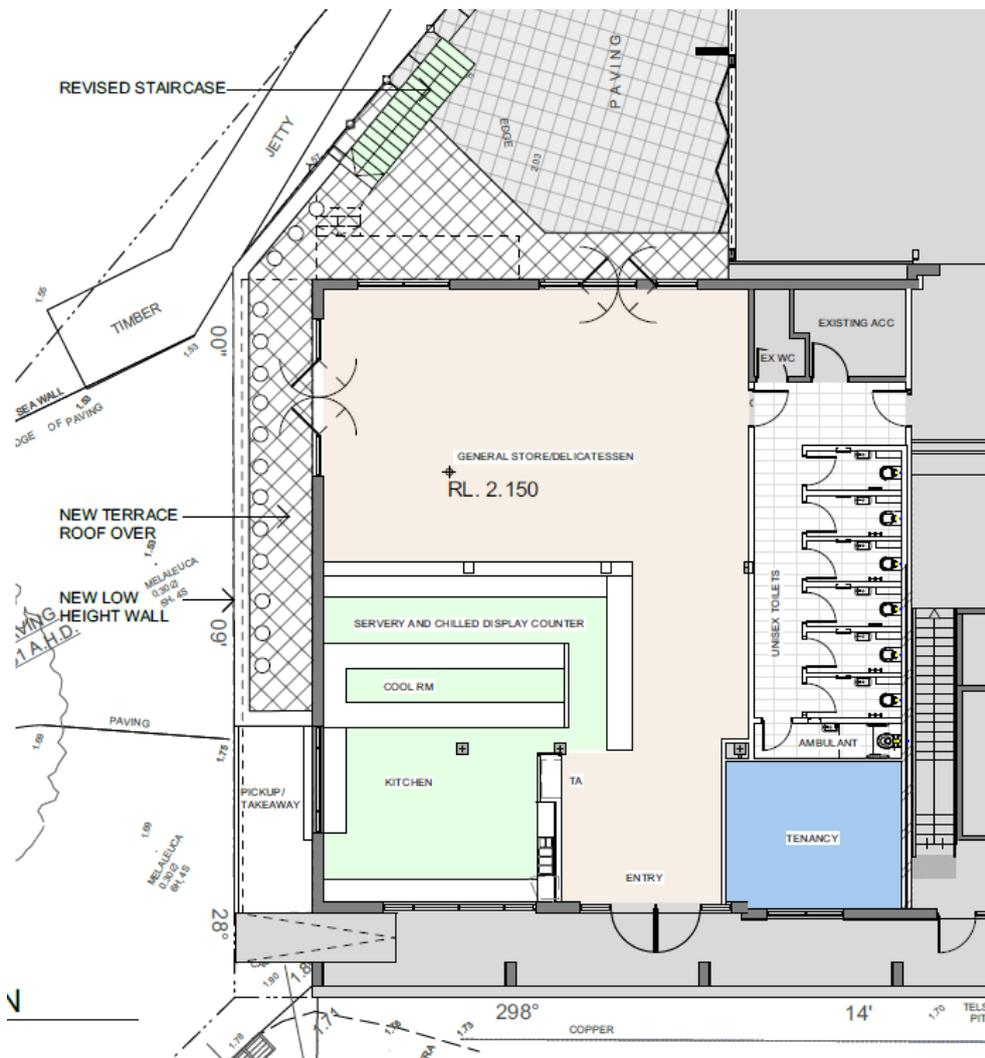
Figure 3 – Proposed new low-height wall and internal modifications
