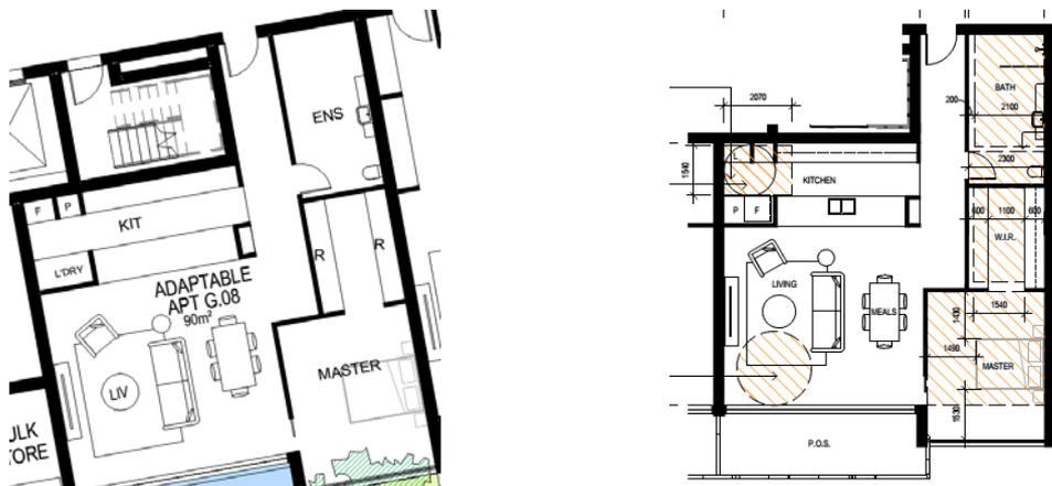
The kitchen does not achieve 1550mm circulation space outside of the kitchen work spaces at post adaptation. This needs to be modified and can be carried out at design development stage.
