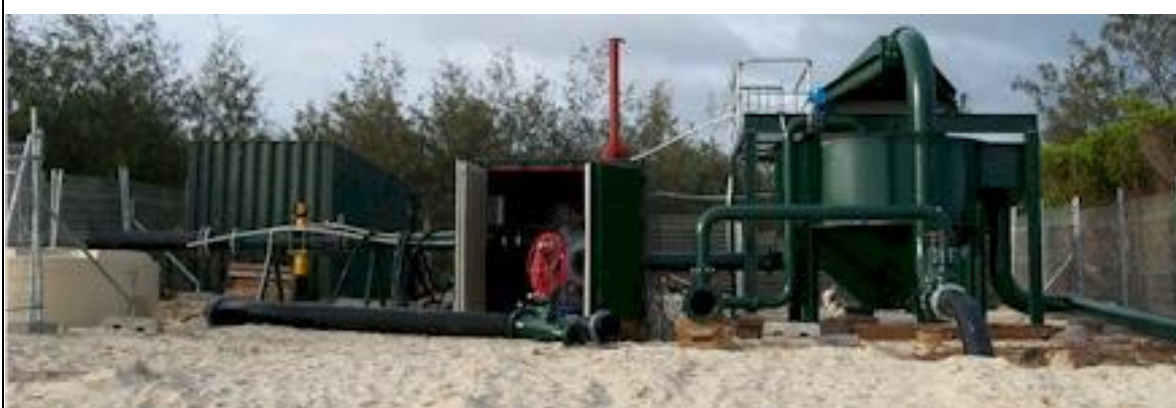
Onshore booster pumps and pipework (Slurry Systems Marine)
