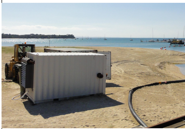
An example pump station as part of operations. Insulated in a shipping container to reduce noise emissions. Photo at Blairgowrie, Vic
