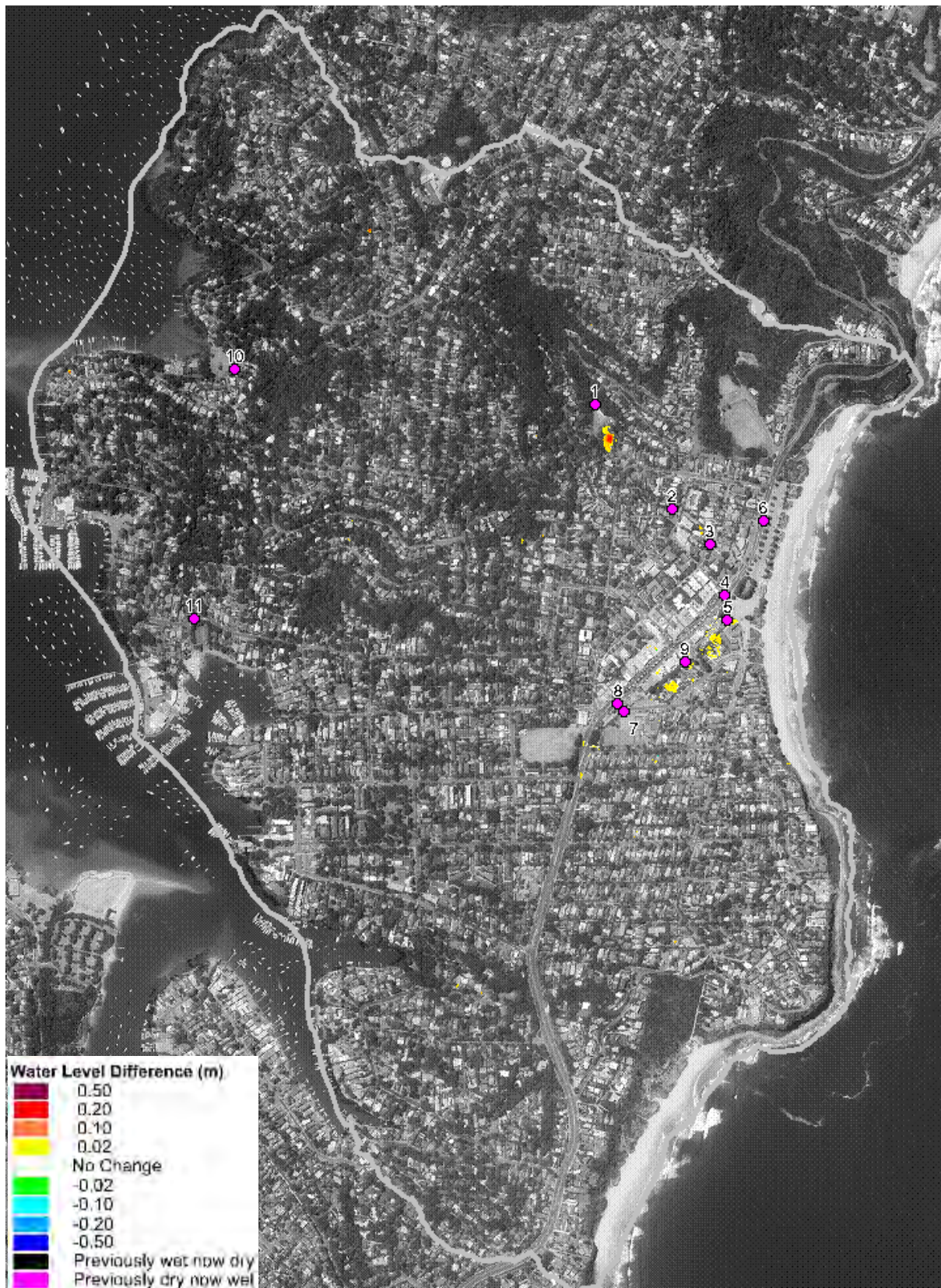
Plate 22 Flood level difference map with reduced continuing loss rates
