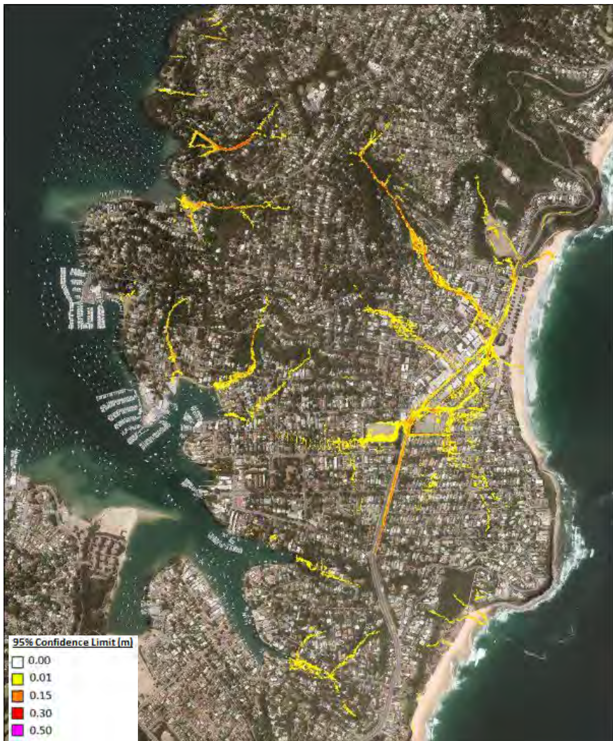
Plate 34 Water level uncertainty grid for other factors that cannot be represented in flood model
