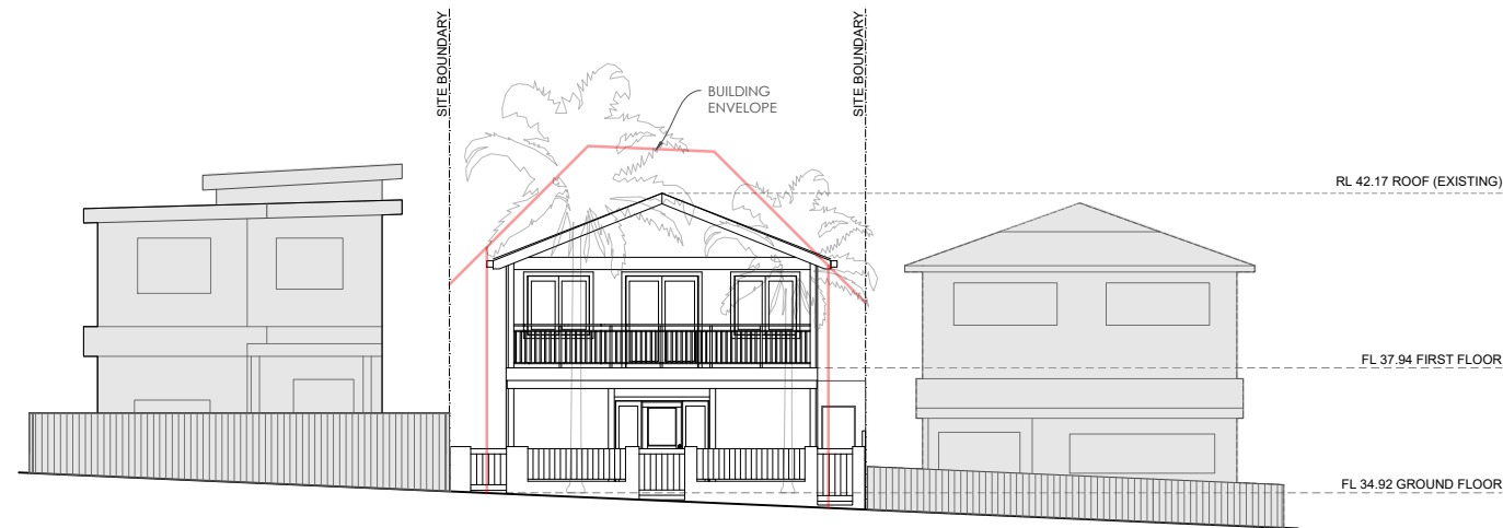
SOUTH ELEVATION (STREET VIEW - JOHNSON STREET)
