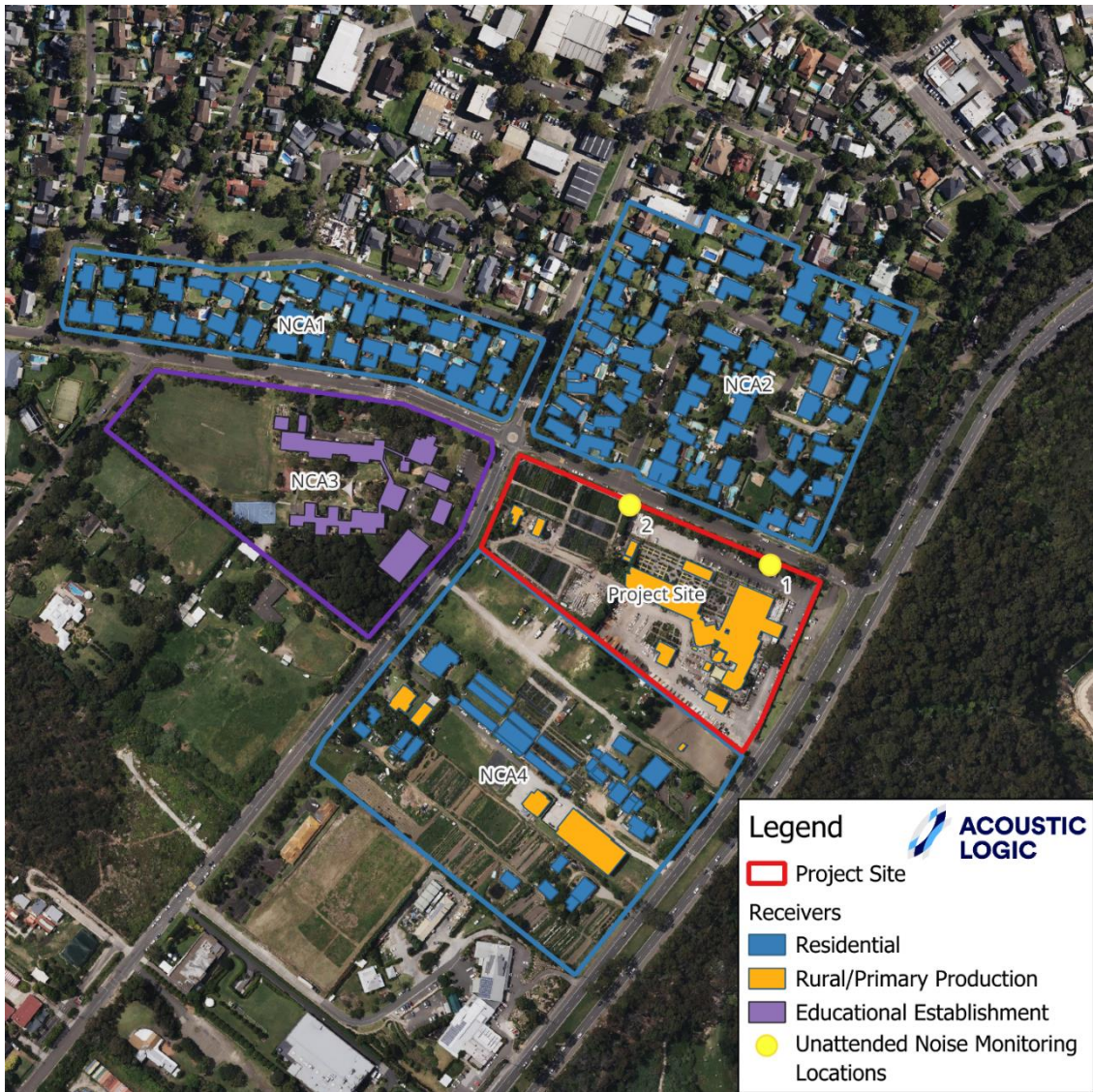
Figure 1 – Site Context and Nearest Sensitive Receivers
