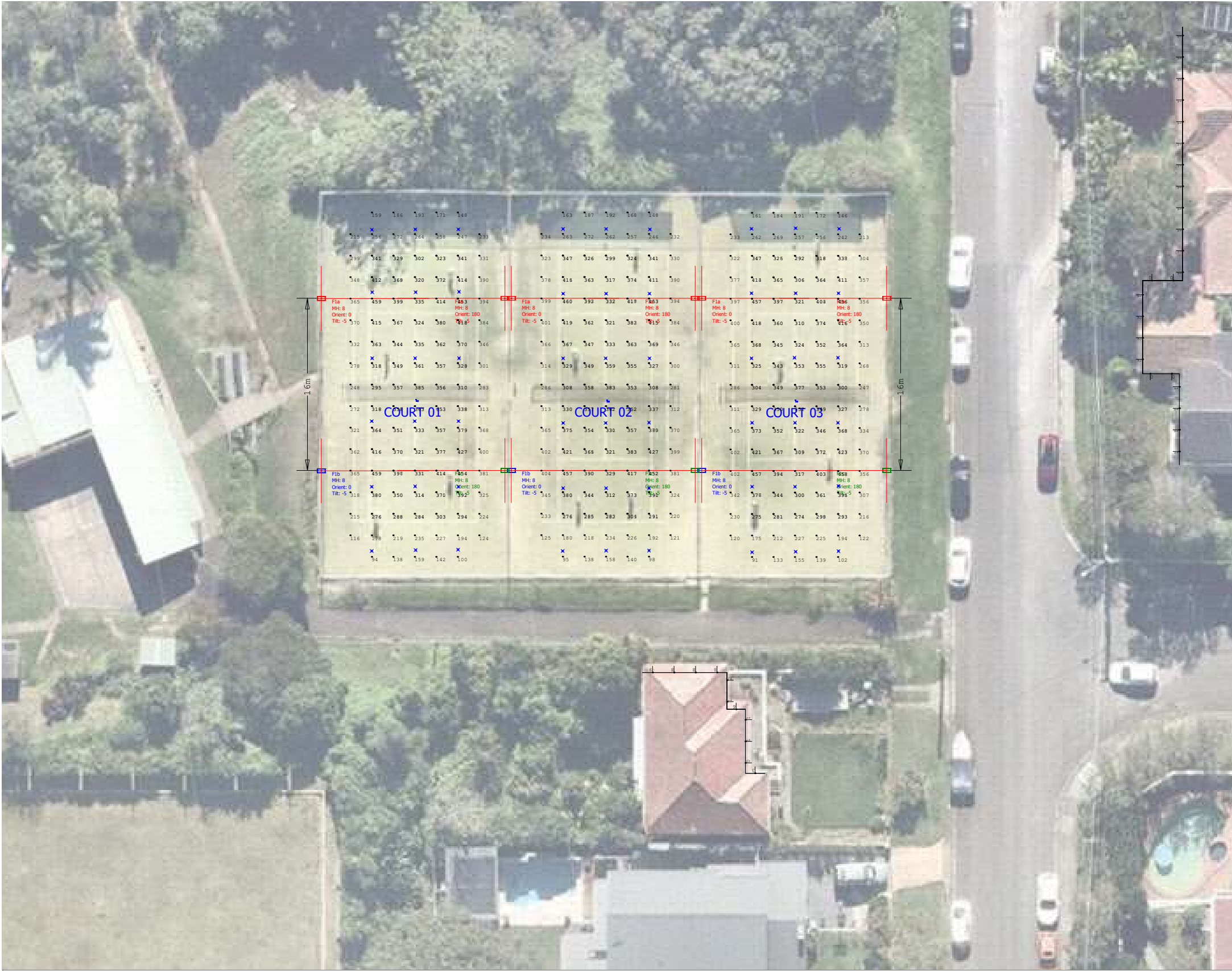
PROPOSED LIGHTING PLAN - Tennis Area 1 Scale= 1: 400
