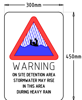
TYPICAL OSD WARNING SIGN DETAIL SCALE: 1:10 @ A3
