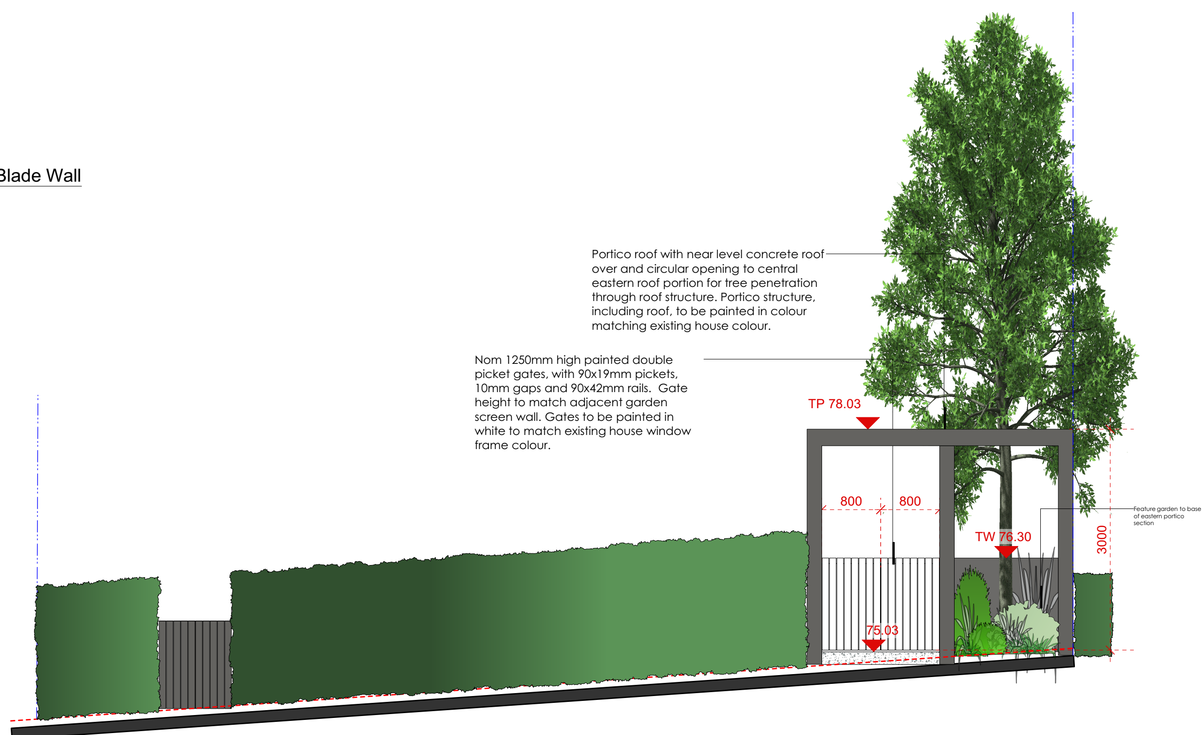
9 Front Boundary Elevation with Proposed Portico Scale: 1:50
