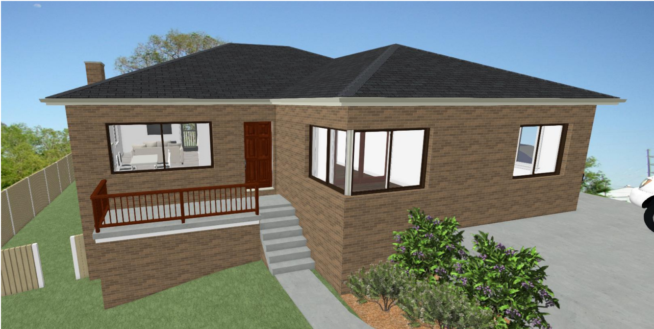
FRONT PERSPECTIVE SHOWING NEW ROOF LINE
