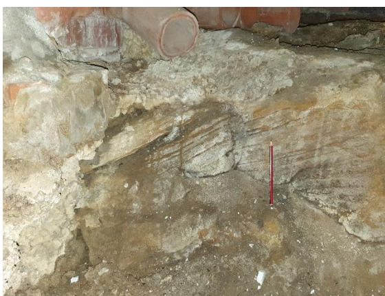
Photograph-2: Bedrock, comprising sandstone of at least low strength with exposed gently north dipping cross bedding defects. View looking east.
