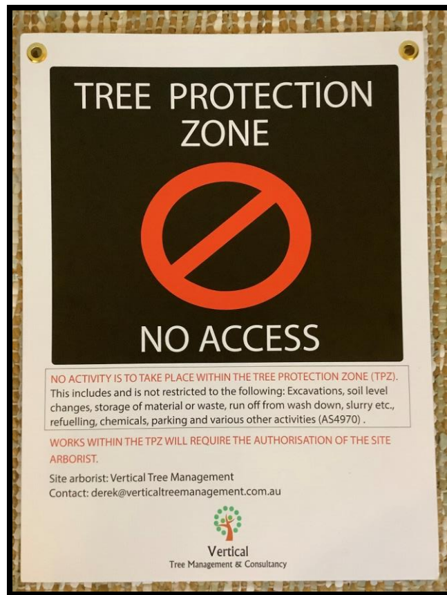
Figure 2 - Tree Protection Signage
