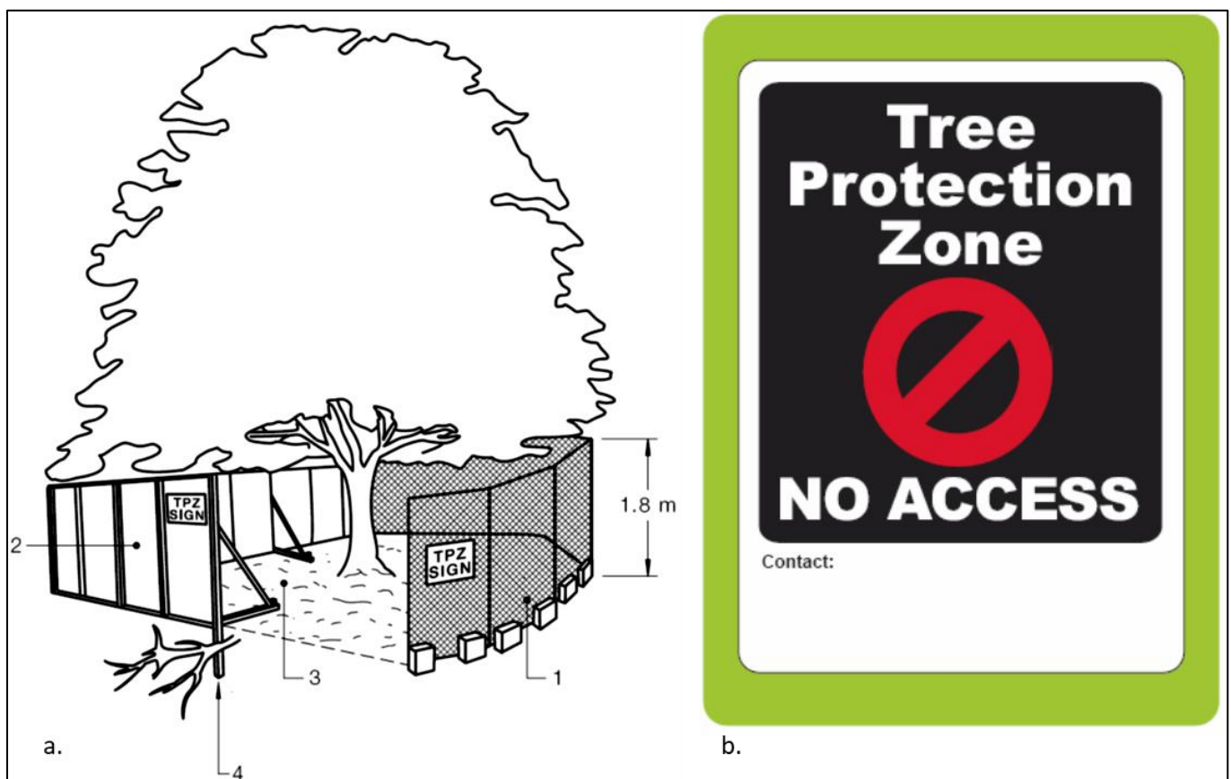
Figure 5. Protection fencing should be erected around the specified perimeter of TPZs in accordance with Section 4.3 of AS4970 (2009) . Figure 11 a. depicts correctly installed steel or plywood fence panelling (1 and 2) with mulch inside the protection area (3). Figure 11 b. shows depicts protection fencing signage.
