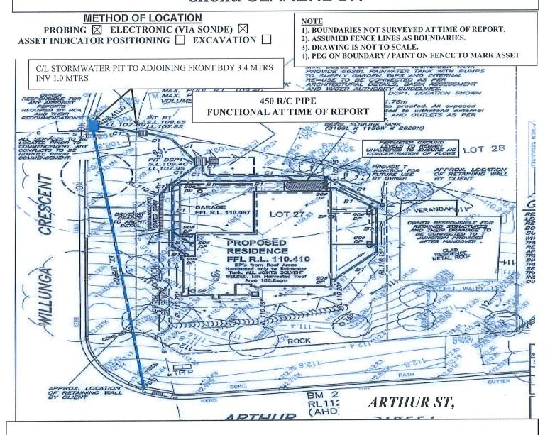
Pipe Size:- 450 MM Pipe Type:- R/C Strata Type:- CLAY / ROCK REFUSAL
