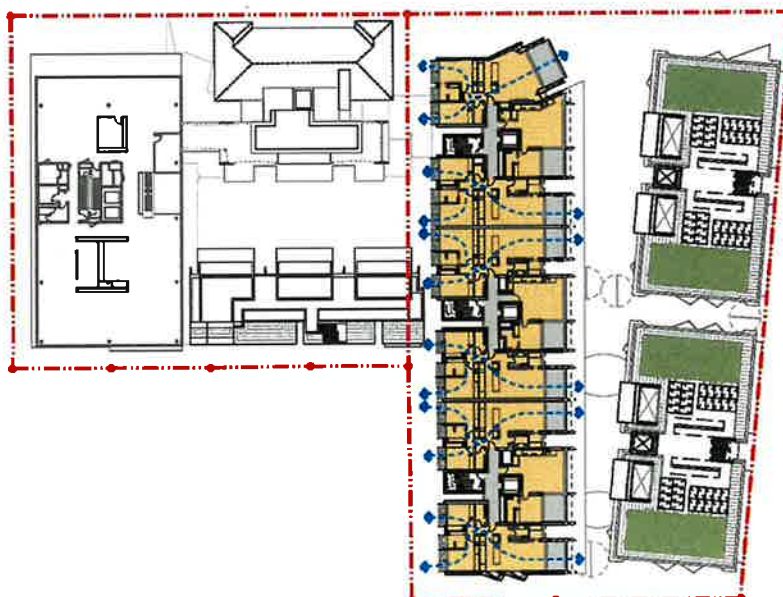
Figure 9: Part plan showing cross ventilation paths through residential apartments on a typical level (Building C).
