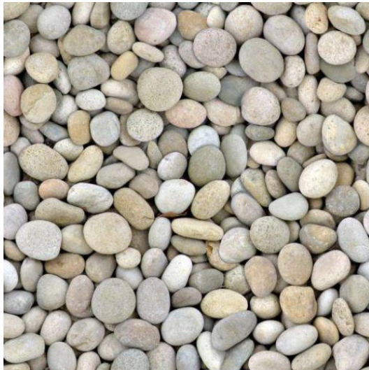
RIVERSTONE PEBBLE BALLAST TO CONCRETE ROOF
