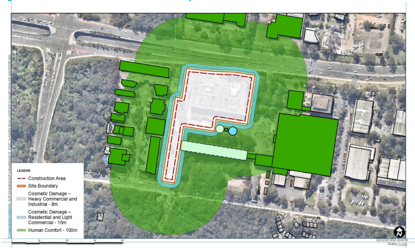
Figure 9 Construction Vibration – 12 T Vibratory Roller
