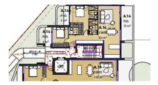
The discharge and path of travel from the northern fire stairs on the ground floor do not comply with D2D12 as is open for less  $\frac{1}{3}$  of its perimeter; and has an unobstructed clear height throughout, including the perimeter openings, of less than 3 m and provides an unimpeded path of travel from the point of discharge to the road or open space of not more than 6 m.
