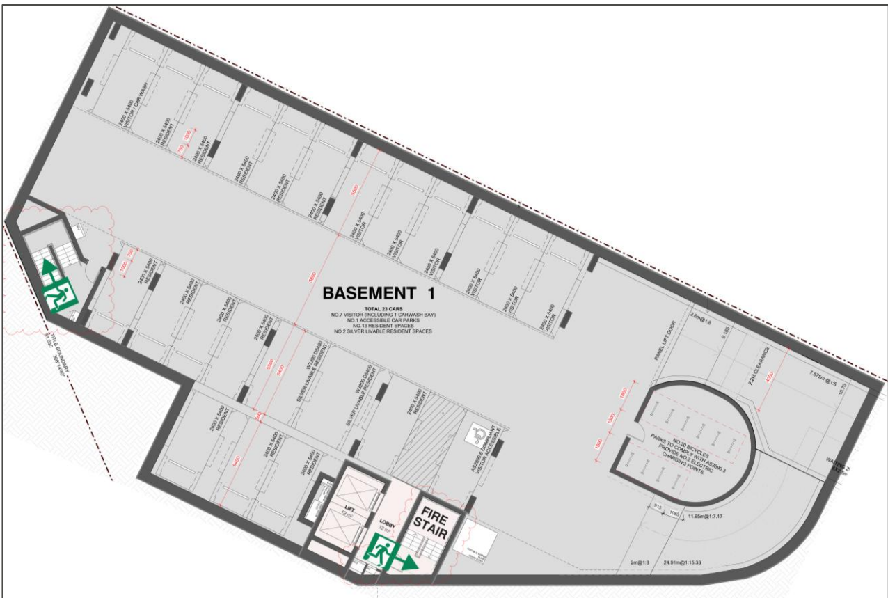
Figure 9: Basement 1 - Exit Locations
