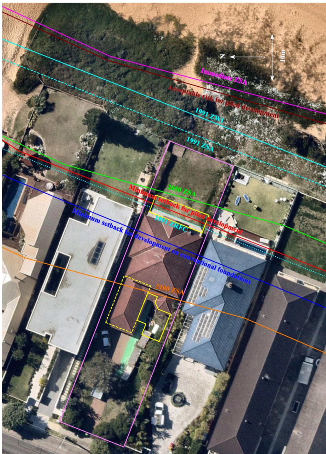
Figure 5: Coastal hazard lines and CZMP setbacks at site, with proposed development outlines in yellow (dashed line shows first floor addition, solid line on seaward side shows deck with pool and spa within this footprint, and solid line on landward side shows ground and first floor addition), and aerial photograph taken on 30 August 2023
