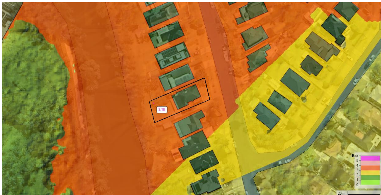
Figure 5 : Pre-Development Water Surface Elevation
