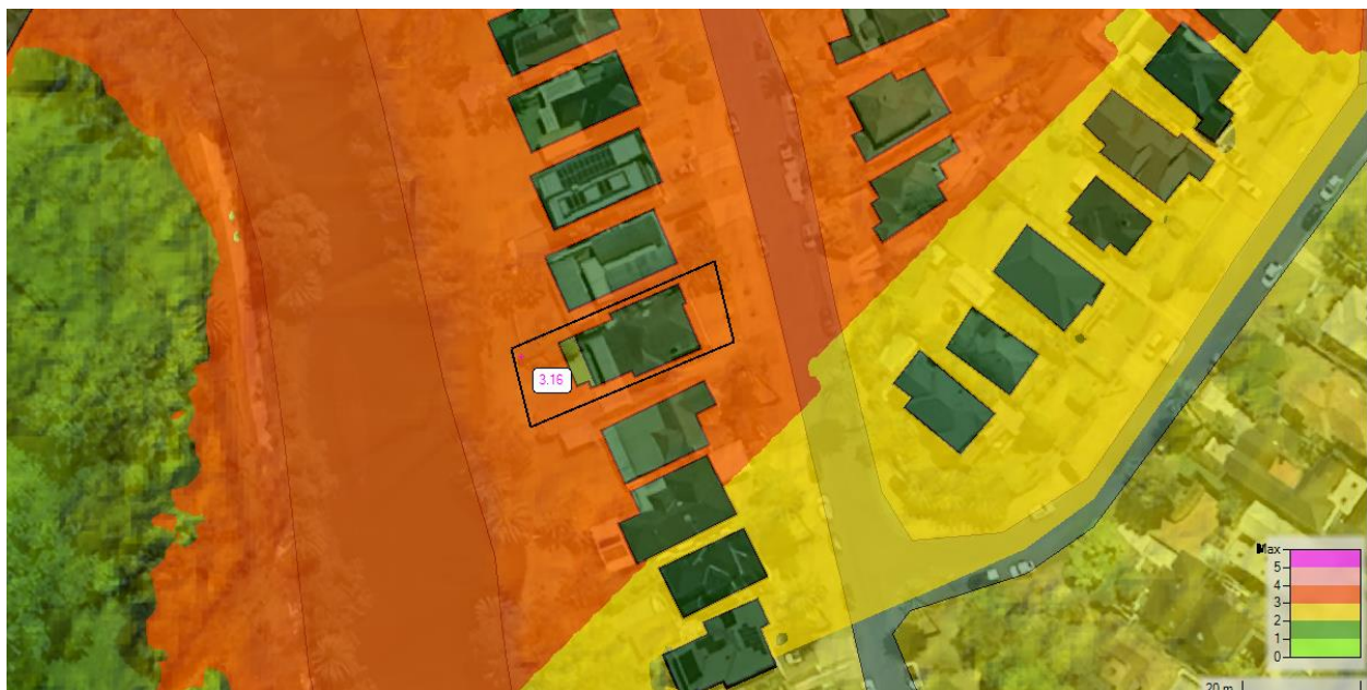
Figure 9 : Post Development Water Surface Elevation
