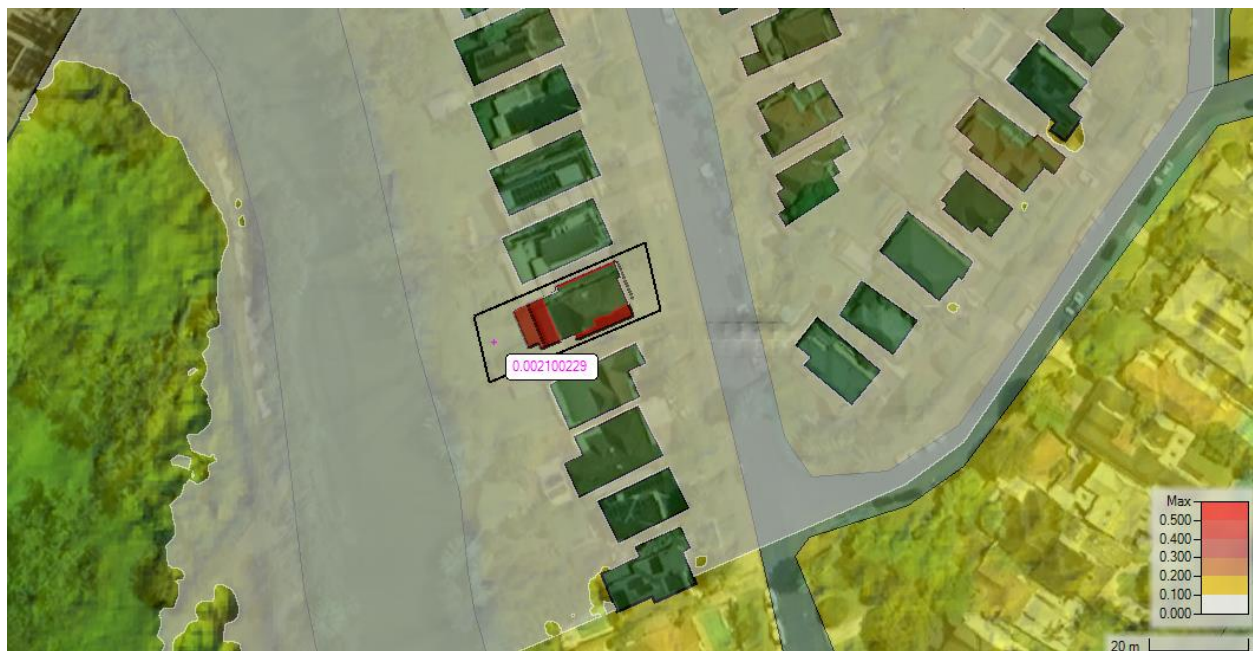
Figure 11 : Graphical comparison of WSE_Postdev-Predev from HEC RAS 2d model.
