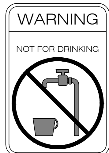
DETAIL 4 RAINWATER SIGN SCALE 1:10
